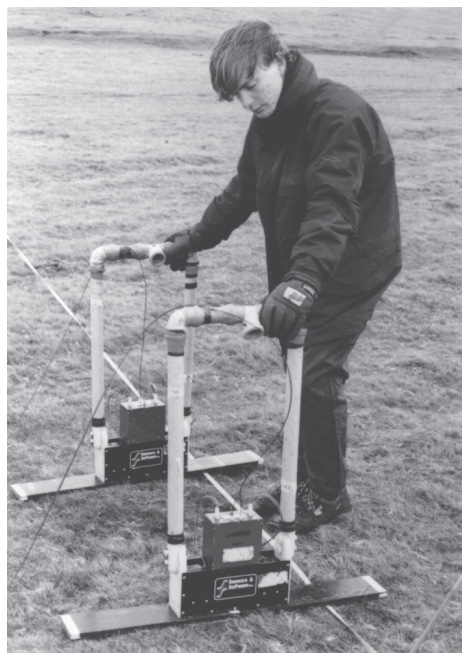
Figure 14.24 GPR instrument and ray paths.
