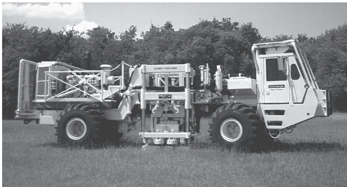
Figure 7.18 A truck for Vibroseis surveying.
